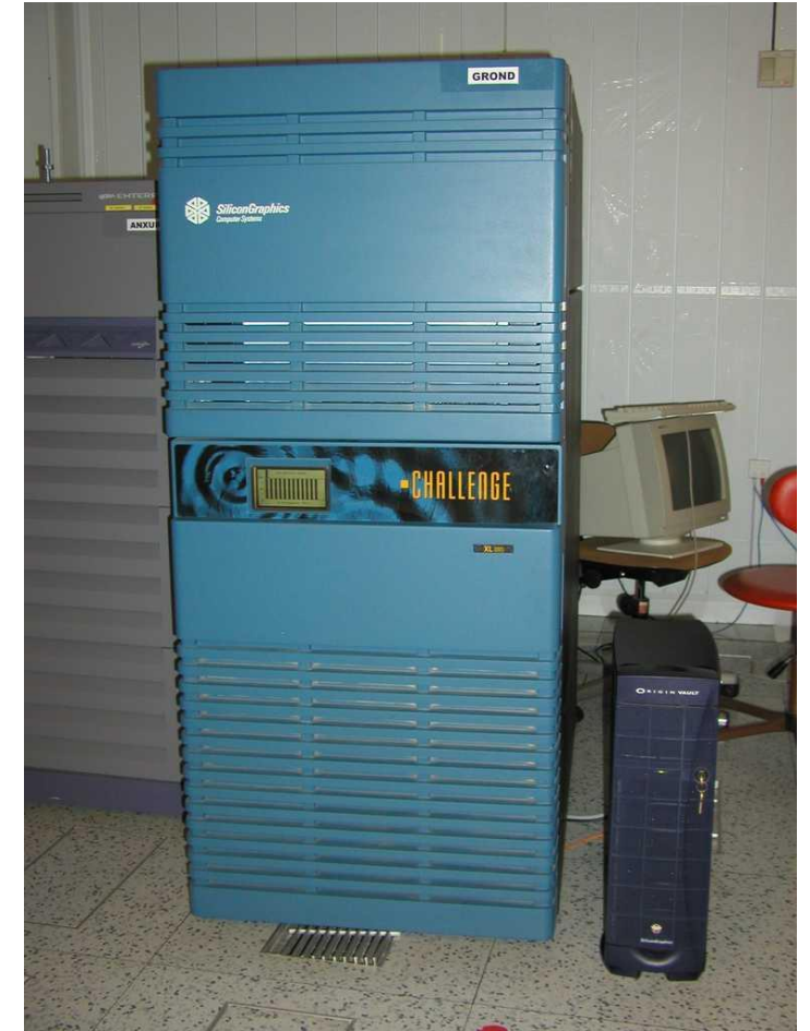
SGI PowerChallenge XL supercomputer with 12 MIPS R10000 processors and 2GB RAM. The first supercomputer at SCB MU. 1994.
